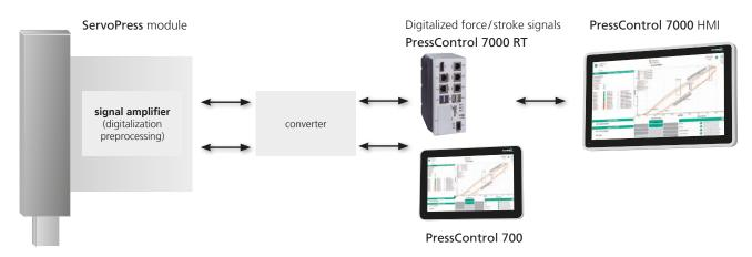
**SCHMIDT® ServoPress/TorquePress** modules operate with a true force control loop (force as a command variable).
