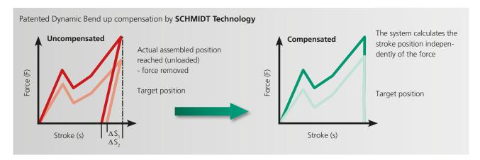
In typical applications, the force required to complete an assembly varies up to 40 % from part to part. When freely positioning, such as without a positive stop, the press ram extends to the same target position, regardless of load. But a closer inspection of the completed assembly and the force/distance curve generated, shows that the final pressed position will vary due to the
