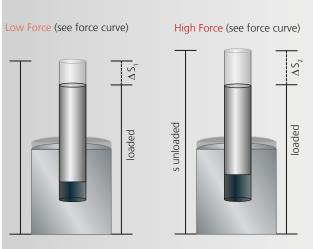
" $\Delta$ S" changes proportionally to the force output, that means, the components have different dimensions depending on the force requirement of each component
