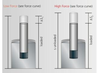
" $\Delta$ S" changes proportionally to the force output, that means, the components have different dimensions depending on the force requirement of each component
