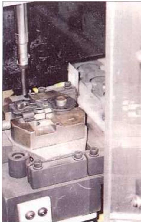
A Schmidt Servo Press with special tooling forces open a spring-operated latch to measure the force and distance needed to push the latch fully down, part of the quality assurance process at latch maker Hatch Stamping.
